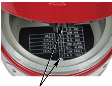
Figure 10—Alignment Guide Location
