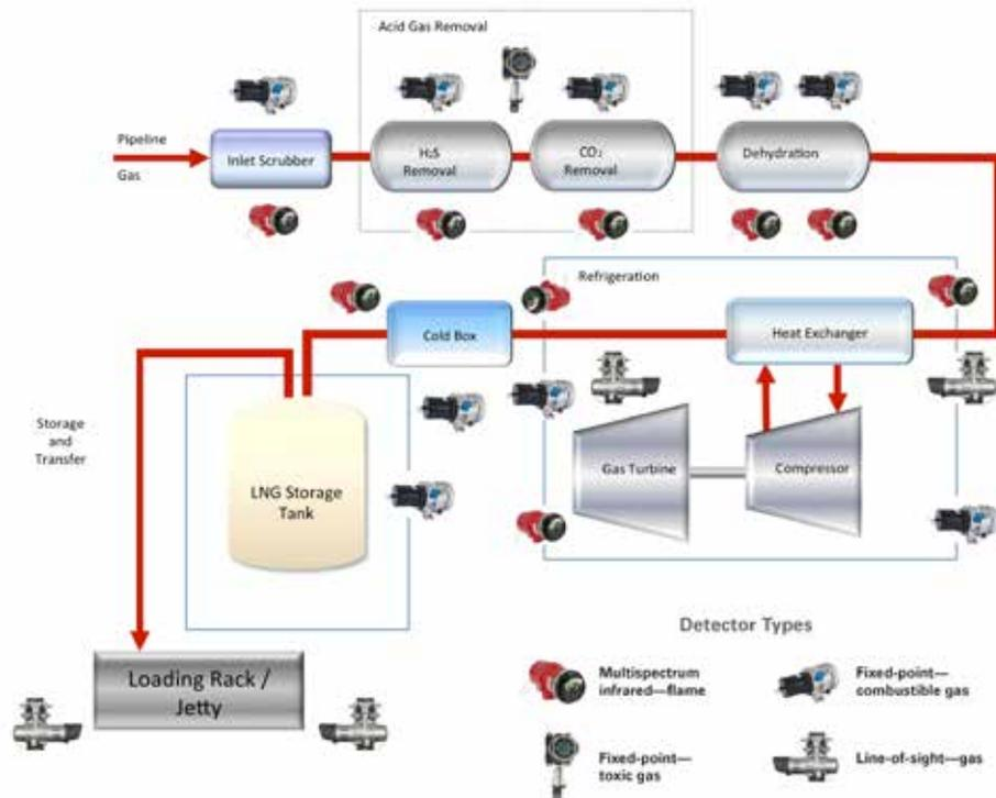
**Figure 2.** This simplified LNG process drawing indicates where detector technologies can be used.
