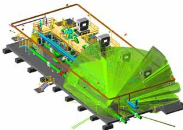
**Figure 1.** 3D mapping can be used to show obstructions in an individual detector's field of view.
