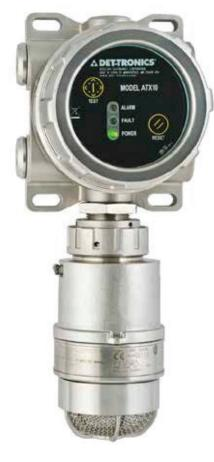
▲▼ Acoustic gas leak detectors work by recognizing the unique sound "fingerprints" of various gases. However, the sound and impact of blowing sand particles can create nuisance ultrasonic noise and lead to possible fault conditions in windy desert environments. The Det-Tronics FlexSonic detector shown above uses a foam filter to eliminate ultrasonic noise due to particle impact with the microphone.
