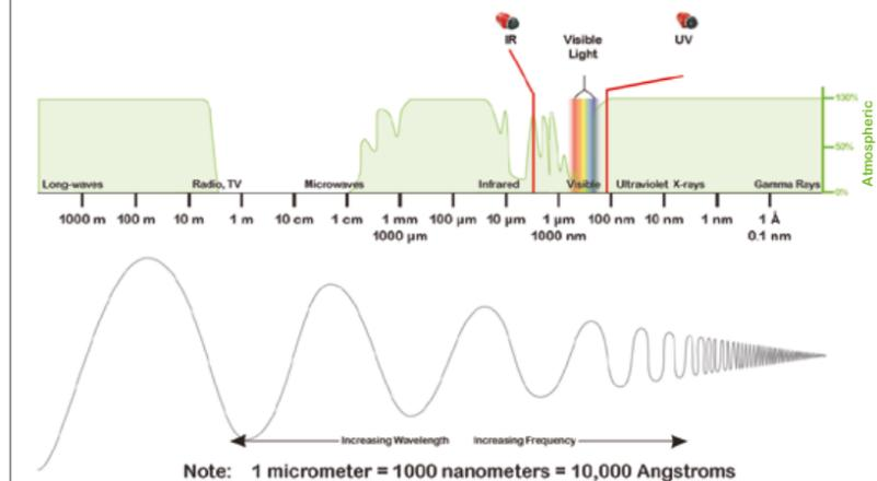
Figure 2 – A broad view of the electromagnetic spectrum depicting the infrared (IR) and ultraviolet (UV) regions that are favourable for the detection of flame
