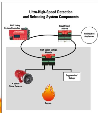
Figure 4 - An example of today's ultra-high-speed flame detection and releasing systems
