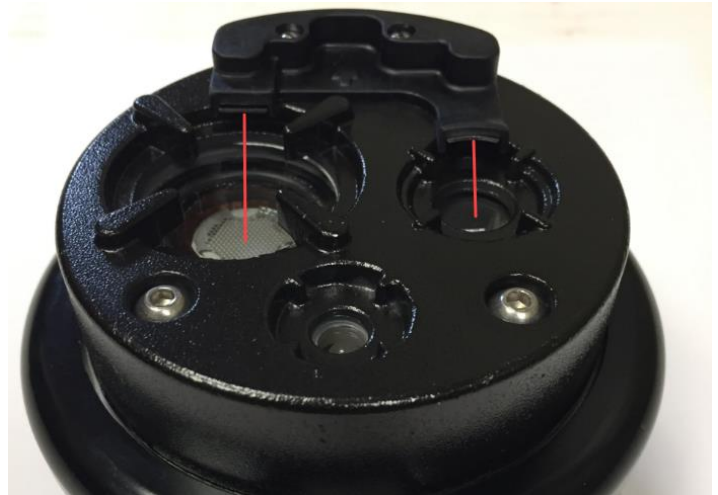
Figure 10: Dramatization of the X5200 UVIR optical integrity signal
