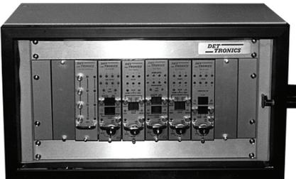
**Enclosure containing R7404 controller, R1425 detonator, R6006 relay module**
