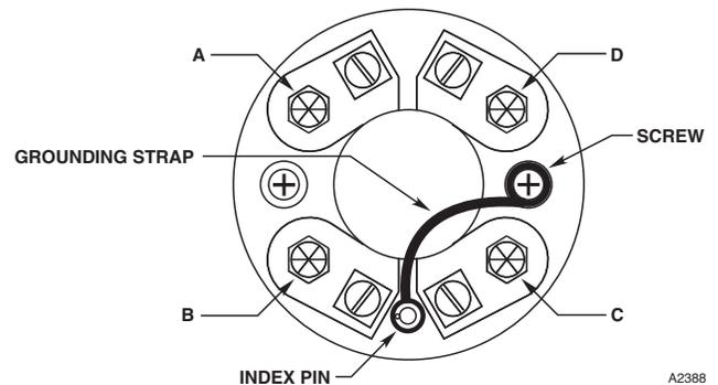
Figure 1—xWatch Terminal Block
