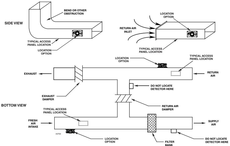
NOTE: WHEN POSSIBLE, THE DETECTOR SHOULD BE LOCATED DOWNSTREAM FROM ANY DUCT OPENING, SHARP BENDS, DEFLECTION PLATES OR BRANCH CONNECTIONS. IF A LOCATION OPTION IS NOT POSSIBLE, LOCATE THE DETECTOR AS FAR AS POSSIBLE FROM THE OPENING, BENDS, DEFLECTION PLATES, ETC.
