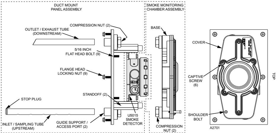
Figure 4—Parts of the Q5016 assembly
