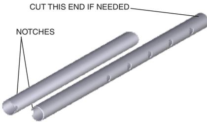
Figure 8—Outlet and inlet tube notches
