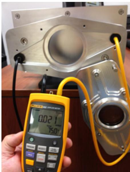
Figure 12—Manometer measurement example
