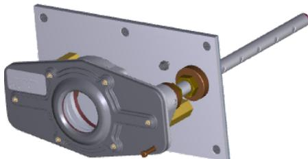
The length of the inlet tube is determined by the width of the duct to be monitored. The inlet tube should span the entire width of the duct. Select the shortest inlet tube that exceeds the width of the duct to be protected. It can then be cut to the exact length during installation.
