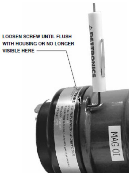
Figure 1— Removing the Sensor Module
