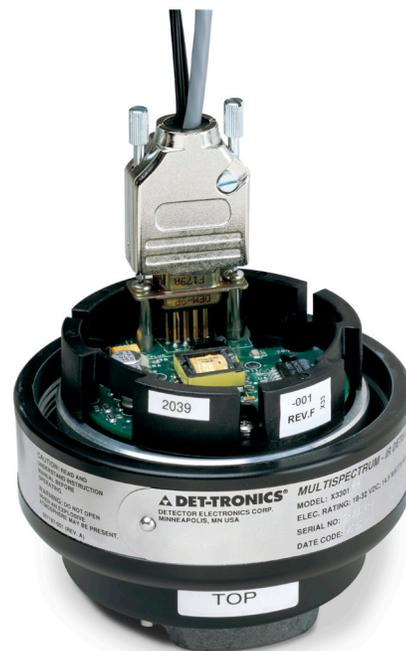
Figure 3—Connecting Inspector Connector to sensor module
