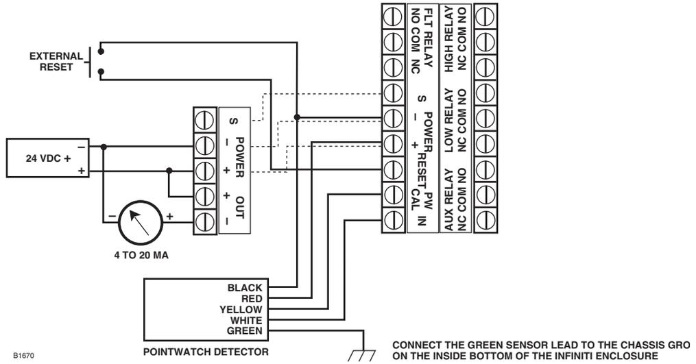
Figure 9—A Typical System - Infiniti Transmitter with a PointWatch Detector and Non-Isolated Current Output
