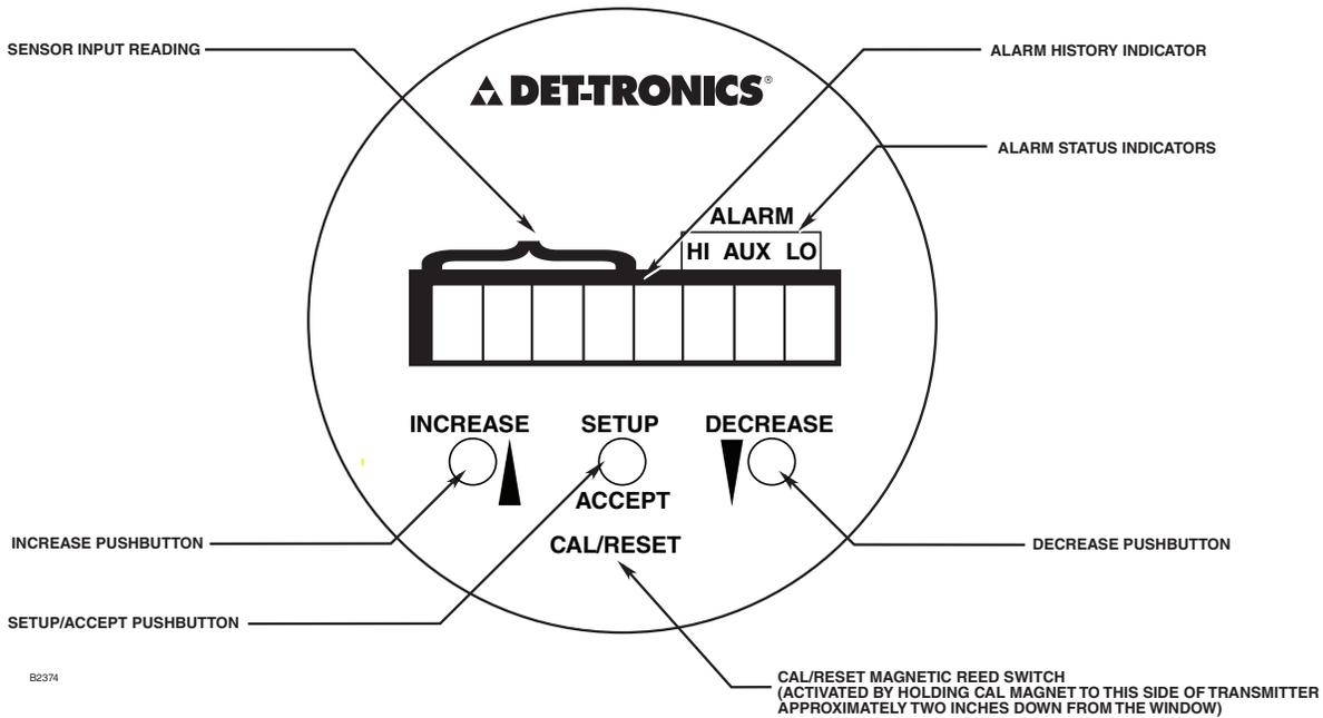
Figure 18—Infiniti Transmitter Controls and Indicators
