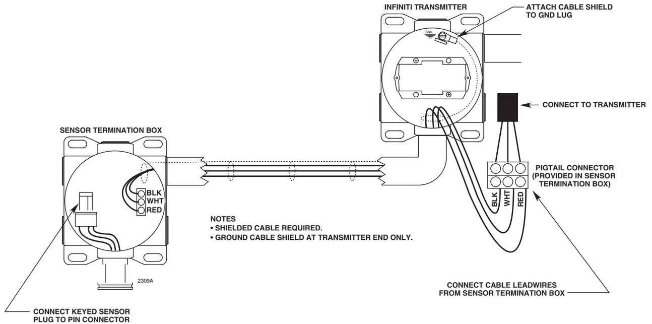
Figure 14—Sensor Separation with Combustible Gas Sensor and Infiniti Transmitter
