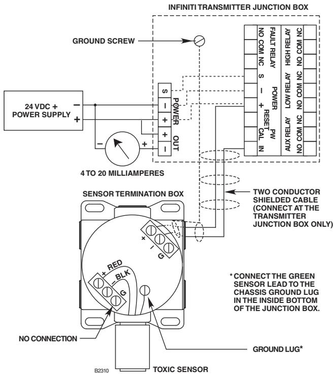
Figure 16—Sensor Separation with Toxic\* and Oxygen Gas Sensors and Infiniti Transmitter
