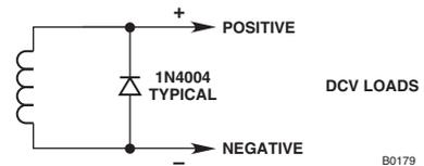
Figure 6—Transient Suppression for Inductive Loads
