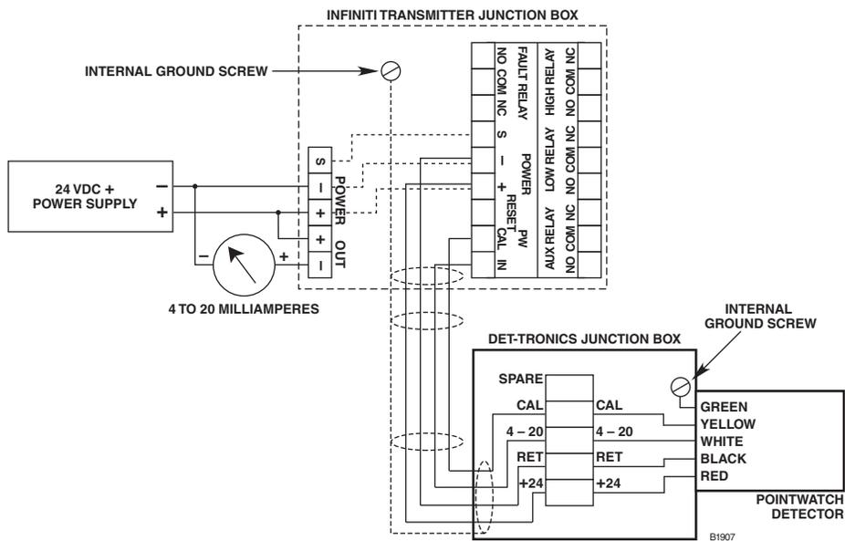
Figure 15—Sensor Separation with PointWatch and Infiniti Transmitter
