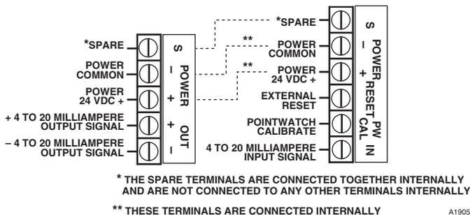
Figure 5—Field Wiring Terminals, Transmitter without Relays
