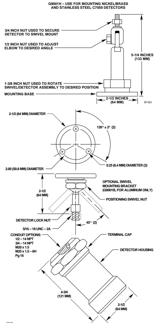
Figure 4—Detector Dimensions in Inches (Millimeters)
