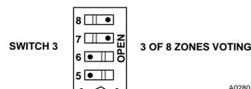
Figure 17—Fire Logic Setting
