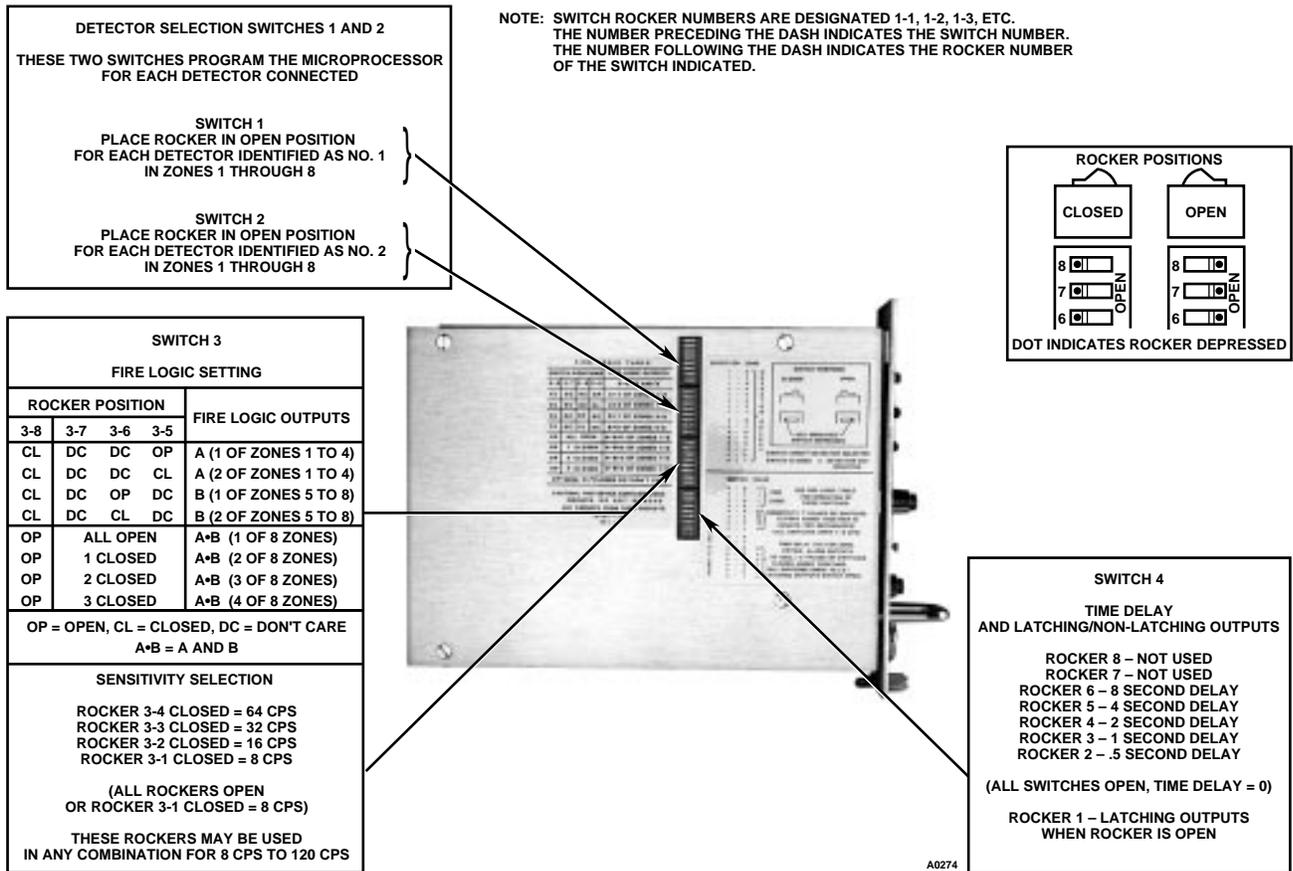
Figure 13—Rocker Switches
