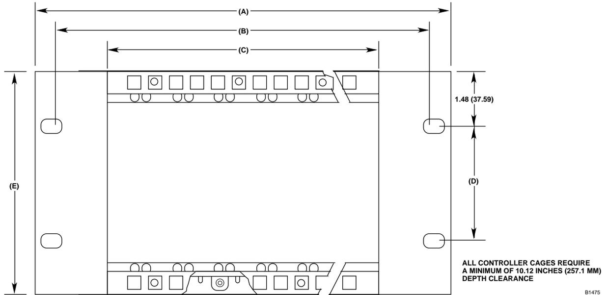
Figure 5—Q4004 Mounting Cage Dimensions in Inches (Millimeters)
