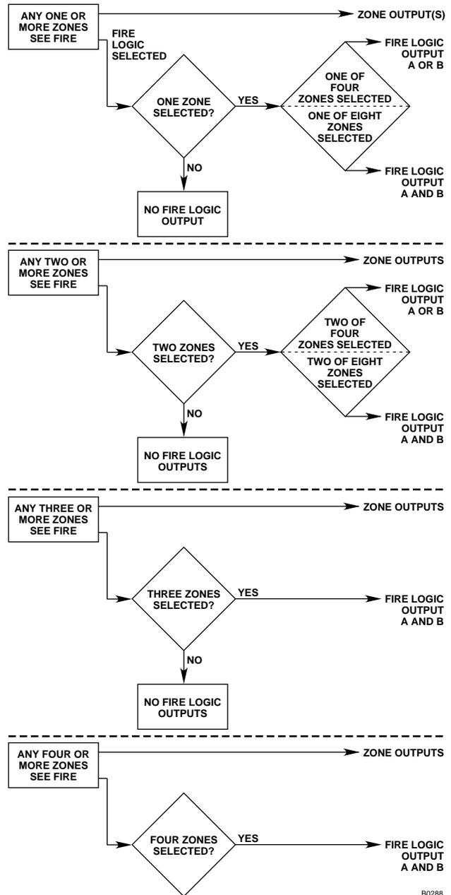
Figure 16—Fire Logic Flow Chart
