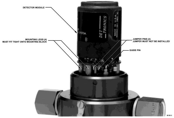
Figure 17—Detector Module Mounting
