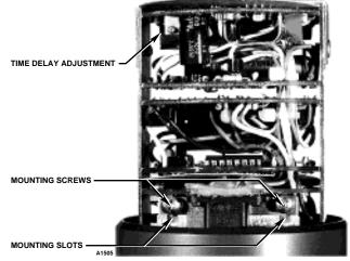
Figure 19—Controller Module Showing Time Delay Adjust
