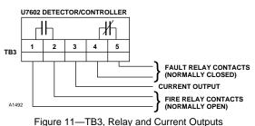
figure 11—TB3, Relay and Current Outputs for Standard Controller Module
