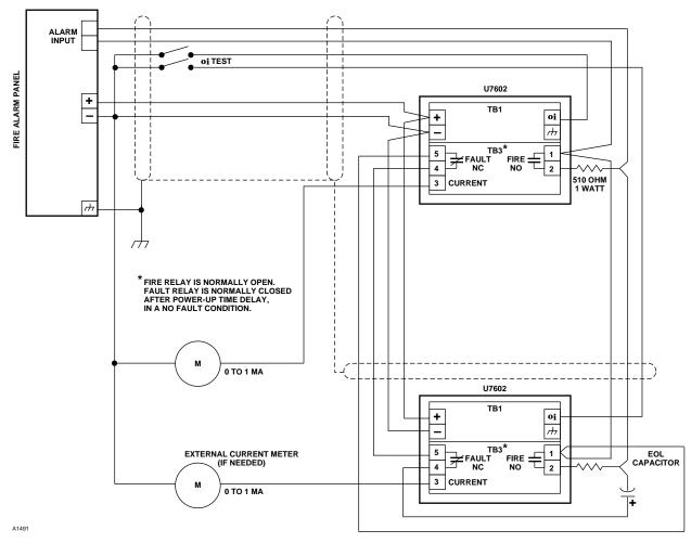
Figure 15—Typical Multiple Unit Configuration with End of Line Capacitors
