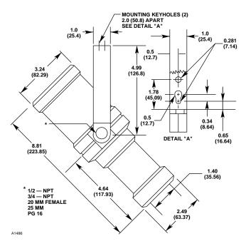
Figure 7—U7602 Dimensions in Inches (Millimeters)
