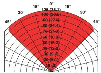
Field of View of X3301 at Indicated Distance in Feet for Methane
