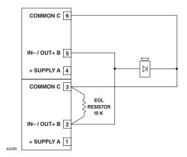
Figure 12—Supervised Output Configuration (Notification)— Class A
