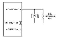
Figure 11—Supervised Output Configuration (Notification)— Class B
