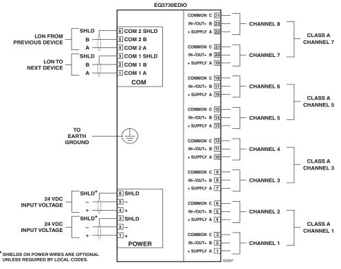
Figure 2—EDIO Module Wiring Terminals
