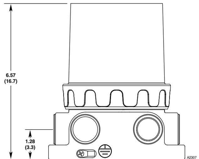
Figure 3—Dimensions of IDCGF in Inches (Centimeters)
