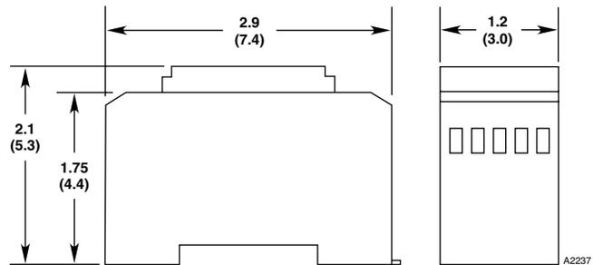
Figure 4—Dimensions of Ground Fault Monitor in Inches (Centimeters)
