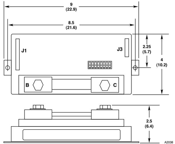
Figure 2—Dimensions of Power Supply Monitor in Inches (Centimeters)
