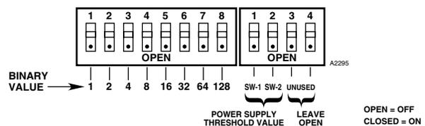
**NOTES:** SWITCHES 1-8 SELECT THE LON ADDRESS. DEVICE ADDRESS EQUALS THE ADDED VALUE OF ALL CLOSED ROCKER SWITCHES.
