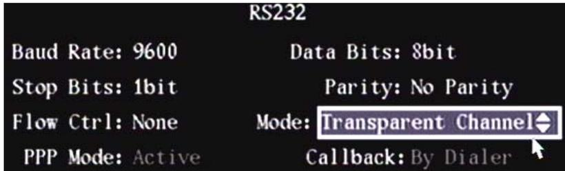
Software must be used in the ATM machine and a command must be sent to the DVR through the RS-232 port based on the manufacturer's communication protocol.
