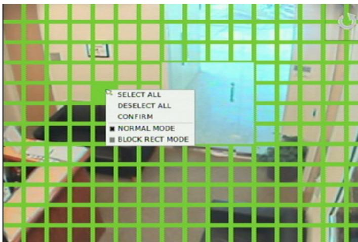
Alternatively, you can select the entire area by right-clicking, and then clicking Select All. A grid covers the entire display screen. Click Deselect All to clear the screen from motion detection. Click Block Rect Mode to select or deselect an entire area block.
