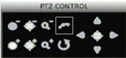
3. Click the Preset icon (or press 1 on the front panel or remote control) to access the Set/Go Preset function as shown in the figure below.
