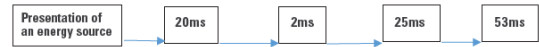
Figure 1: Example of the timeline from detection of an ignition source to releasing the mitigation system.
