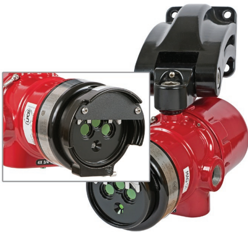
Figure 1: Heavy wind, rain or snow can lead to weather-induced fault conditions for flame detectors because infrared radiation is absorbed by water molecules. To minimize the accumulation of moisture or condensation on detector optics, look for IR detectors with lens heaters and device shielding (as shown on the Det-Tronics X3301 Multispectrum IR detector above).
