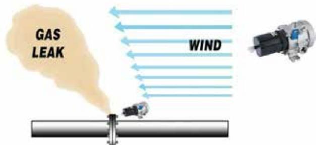
**Figure 3.** Covering a hazard area with voting detectors can reduce the probability of alarming in the face of a legitimate threat, particularly where environmental factors such as wind may be present.
