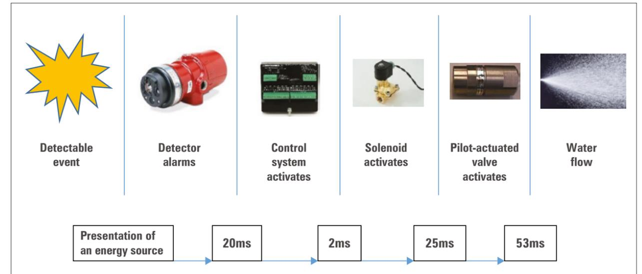
Figure 3b – Per NFPA 15, Standard for Water Spray Fixed Systems for Fire Protection, response time for an entire ultra-high-speed detection and suppression system from presentation of an energy source at the detector to flow of water from the water spray nozzle cannot exceed 100 milliseconds (ms).
