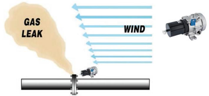
**Figure 2:** Covering a hazard area with voting detectors can reduce the probability of alarming in the face of a legitimate threat, particularly where environmental factors such as wind may be present.
