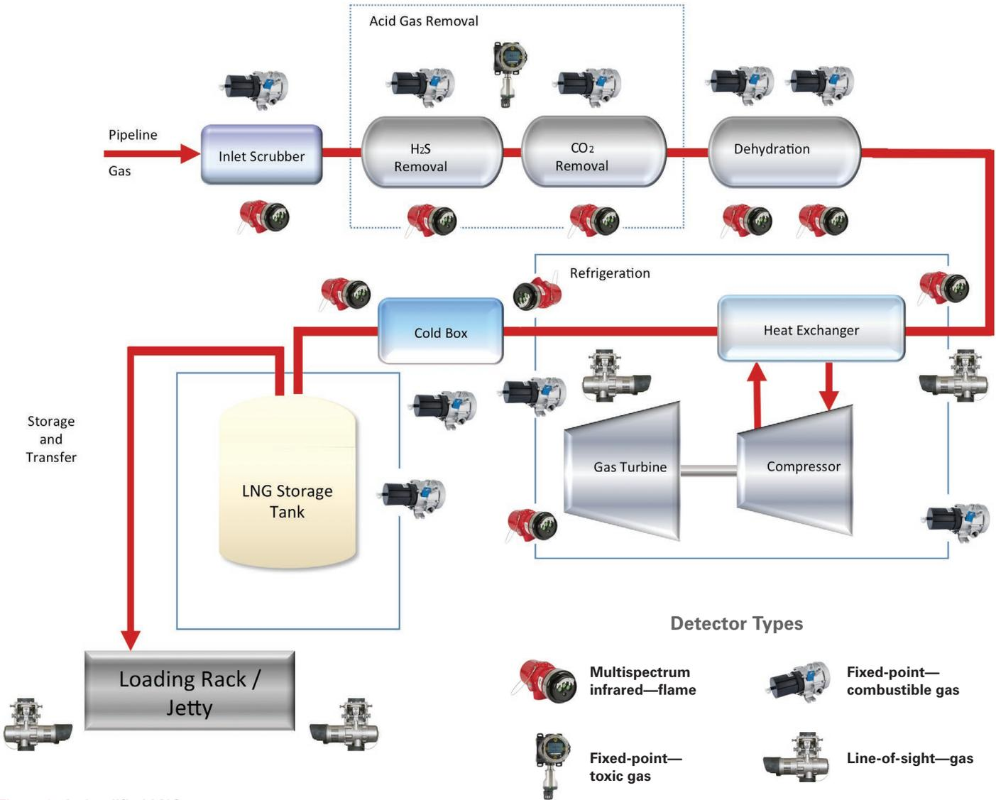
**Figure 3: A simplified LNG process**
