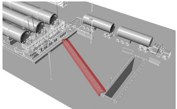
**Figure 4: Offloading and storage areas in LNG facilities also require coverage by flame and gas detectors. The diagrams depict three typical hazard zones: an emergency impounding basin, the storage tank process area and a cross-site transfer trench.**
