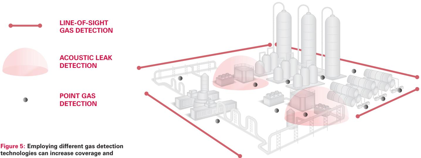
**Figure 5: Employing different gas detection technologies can increase coverage and reduce risk in high-hazard environments such as LNG processing facilities.**
