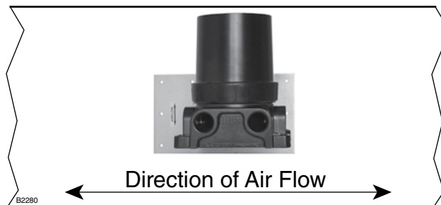
Orientation of PIRDUCT Mounting Plate Relative to Direction of Airflow through Duct
