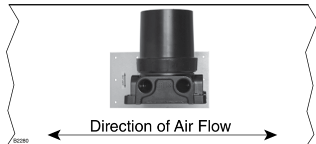
Orientation of PIRDUCT Mounting Plate Relative to Direction of Airflow through Duct
