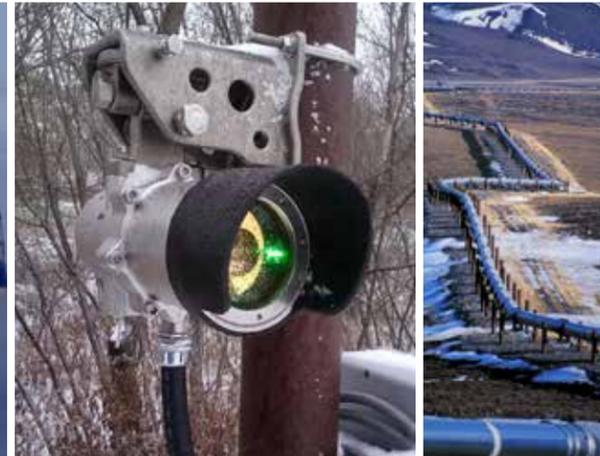
Det-Tronics FlexSight™ LS2000 line-of-sight infrared gas detector is third-party certified and is SIL 2 capable.
