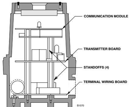
Figure 3-55—Printed Circuit Boards in Combustible Gas DCU
