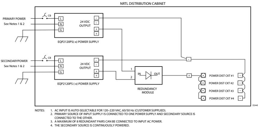
Figure 3-21A—Wiring Connections for a 20amp DC (Maximum) Power Supply with Primary and Secondary AC Sources
