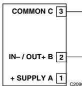
Figure 3-24—Unsupervised Input Configuration
