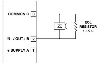
Figure 3-32—Supervised Output Configuration (Notification)— Class B
