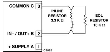
Figure 3-27—Supervised Input Configuration for Opens and Shorts – Class B
