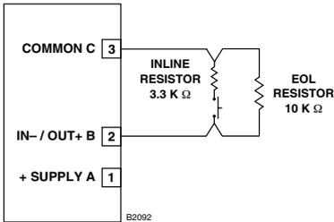
Figure 3-40—Supervised Input Configuration (Opens and Shorts)
