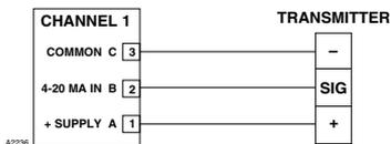
Figure 3-48—Three-Wire Transmitter — Non-Isolated 4 to 20 mA Current Output (Sourcing)
