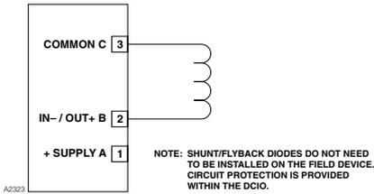
Figure 3-42—Supervised Output Configuration
