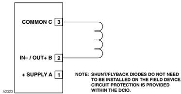
Figure 3-43—Unsupervised Output Configuration
