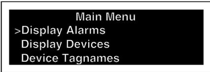
Moving within the Main Menu is done by using the NEXT or PREVIOUS pushbuttons located on the controller's front panel. The menu options will scroll upward (NEXT Pushbutton) or downward (Previous Pushbutton) while the Main Menu name remains stationary. When the desired menu option is selected by the ">" indicator, the ENTER pushbutton is pressed to advance the menu display to the desired information set.
