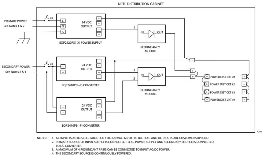
Figure 3-21C—Wiring Connections for a 20amp (Maximum) Power Supply with an AC Primary and DC Secondary Source
