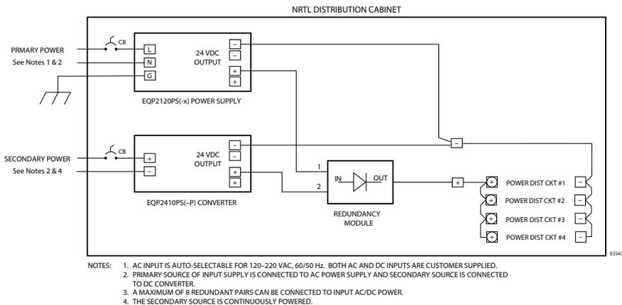
Figure 3-21B—Wiring Connections for a 10amp (Maximum) Power Supply with an AC Primary and DC Secondary Source
