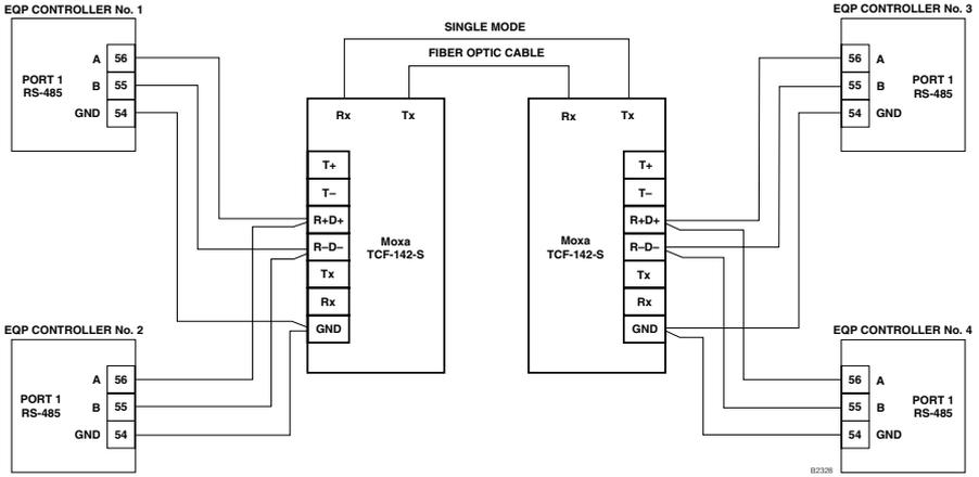
Figure 3-12—Controller to Controller NFPA 72 Approved Fiber Optic Link, Class B
