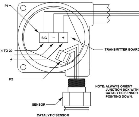
A plug with screw terminals is provided for connecting the cable to P2 on the transmitter board. Observe the wiring color code. Connect the shield to the ground terminal in the DCUEX junction box.
