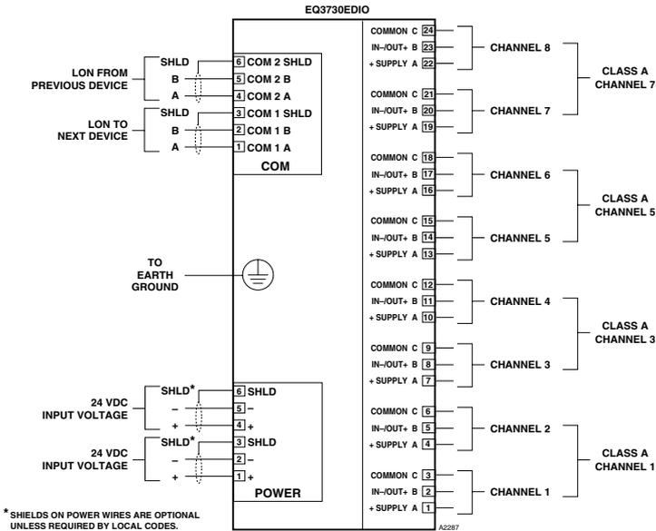
Figure 3-23—EDIO Module Wiring Terminals
