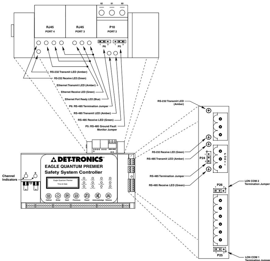
Figure 3-10B—Location of Termination Jumpers, Communication Indicator LEDs, and Communication Ports for Controller with Ethernet Interface Board
