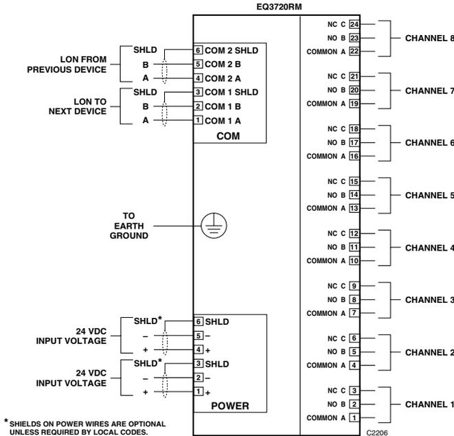
NOTE: RELAY CONTACTS SHOWN IN REST (DE-ENERGIZED) STATE.
