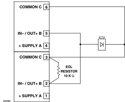
Figure 3-33—Supervised Output Configuration (Notification)— Class A
