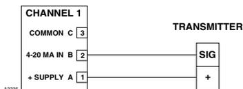
Figure 3-46—Two-Wire Transmitter — Non-Isolated 4 to 20 mA Current Output (Sourcing)
