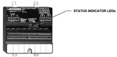
Figure 4-7—DCIO Module Status Indicator Location
