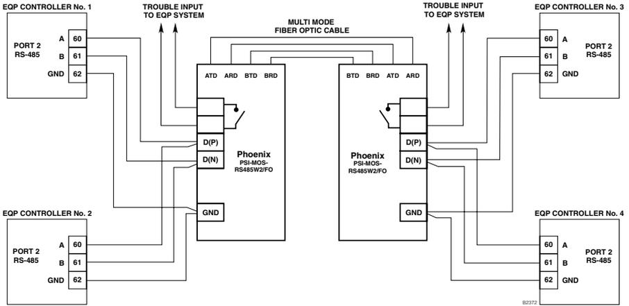
Figure 3-14—Multi-Mode Controller to Controller NFPA 72 Approved Fiber Optic Link, Class X
