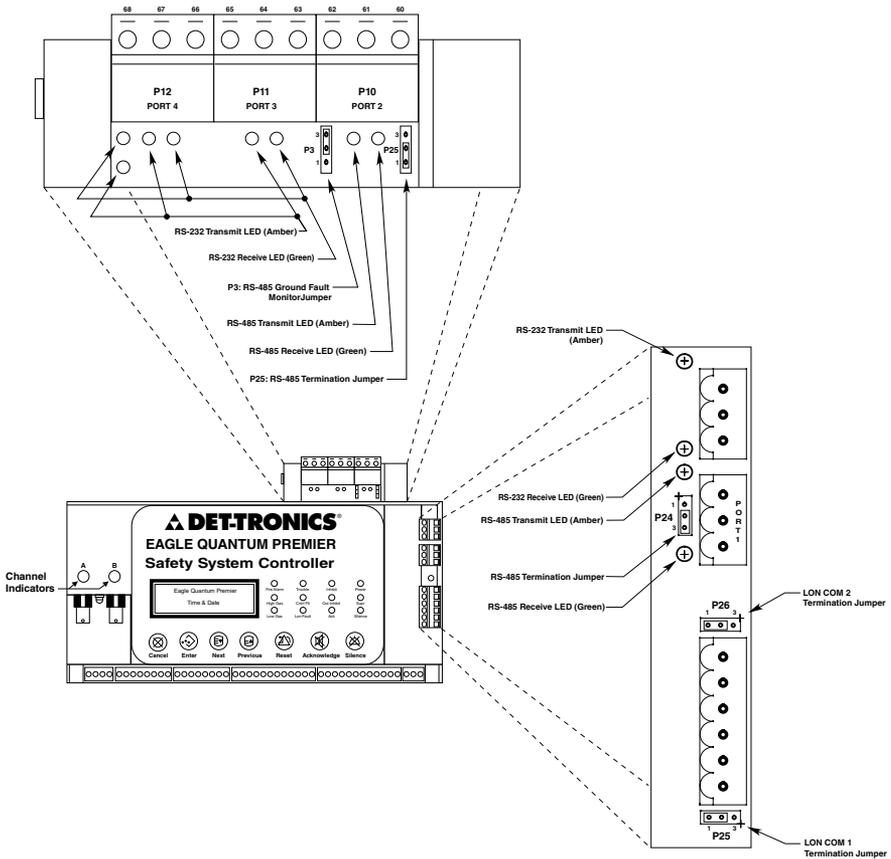
Figure 3-10A—Location of Termination Jumpers, Communication Indicator LEDs, and Communication Ports for Controller with Serial Interface Board
