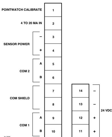
Figure 3-51—Wiring Configuration for DCU
