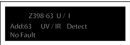
Pressing the NEXT or PREVIOUS pushbuttons allows cycling through devices. Pressing the CANCEL pushbutton will return the display to the Main Menu.
