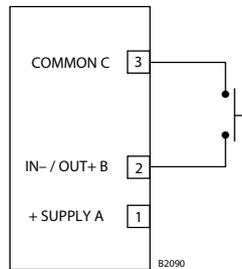
Figure 3-38—Unsupervised Input Configuration
