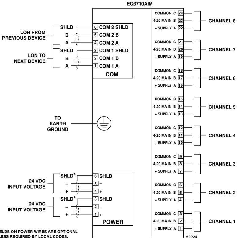
Figure 3-45—Analog Input Module Wiring Terminal Configuration
