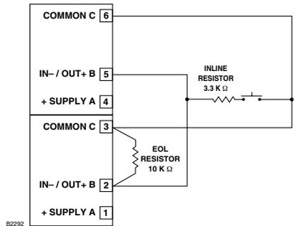
Figure 3-28—Supervised Input Configuration for Opens and Shorts – Class A
