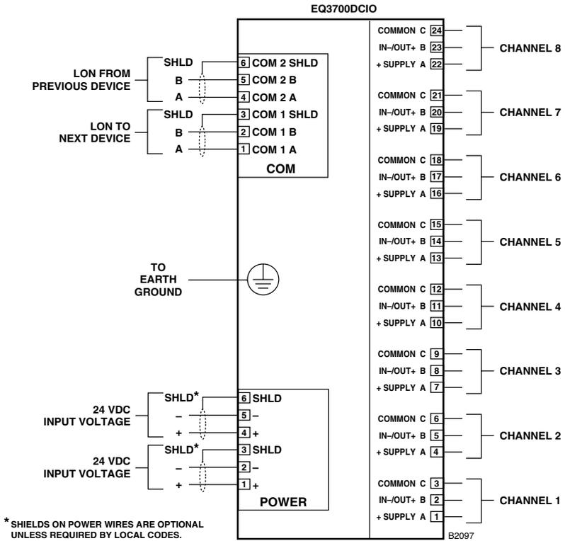
Figure 3-37—DCIO Module Wiring Terminal Configuration
