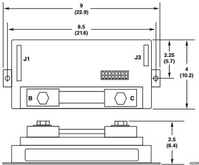
Figure 6-4—Dimensions of Power Supply Monitor in Inches (CM)
