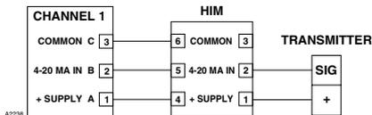
Figure 3-47—Two-Wire Transmitter with HART Interface Module — Non-Isolated 4 to 20 mA Current Output (Sourcing)
