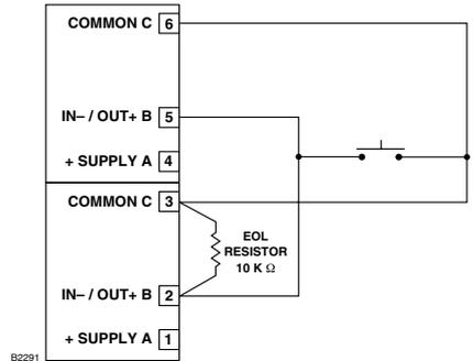
Figure 3-26—Supervised Input Configuration – Class A
