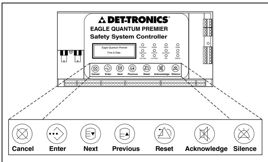
Figure 4-1—EQP Controller Pushbutton Locations
