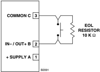
Figure 3-39—Supervised Input Configuration
