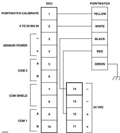
Figure 3-53—PointWatch/DuctWatch Connected to DCU
