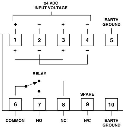
**NOTE:** RELAY CONTACTS ARE SHOWN IN THE REST STATE, NO POWER APPLIED. RELAY IS ENERGIZED WITH POWER APPLIED AND NO GROUND FAULT (TERMINALS 6 & 7 CLOSE, TERMINALS 6 & 8 OPEN).
