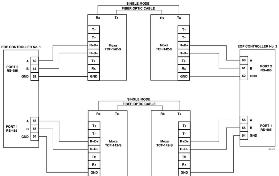
Figure 3-13—Single Mode Controller to Controller NFPA 72 Approved Fiber Optic Link, Class X
