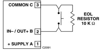
Figure 3-25—Supervised Input Configuration – Class B
