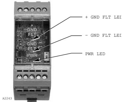
Figure 4-11—Ground Fault Monitor Status Indicator Location
