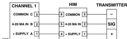
Figure 3-49—Three-Wire Transmitter with HART Interface Module — Non-Isolated 4 to 20 mA Current Output (Sourcing)
