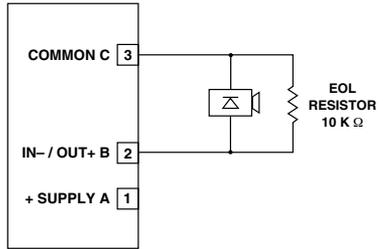
Figure 3-41—Supervised Output Configuration (Notification)
