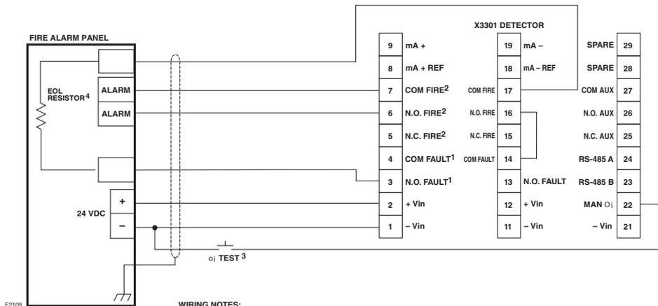
Figure 8—Ex d e Wiring Option
