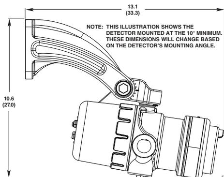
Figure 3—Q9033 Mounting Arm without Collar Attachment Dimensions in Inches (cm)
