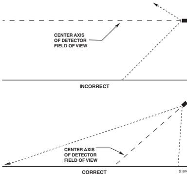
Figure 1—Detector Orientation Relative to Horizon
