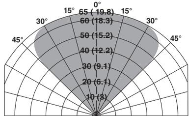
Field of View at Indicated Distance in Feet (m) for **Methane** at **Medium** Sensitivity (30 inch plume)
