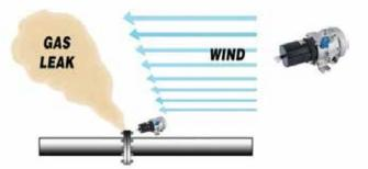
**Figure 3.** Covering a hazard area with voting detectors can reduce the probability of alarming in the face of a legitimate threat, particularly where environmental factors such as wind may be present.
