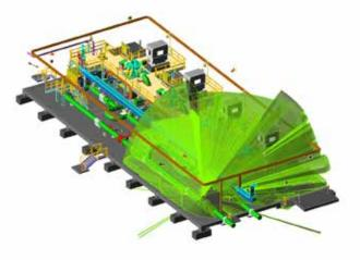
**Figure 1.** 3D mapping can be used to show obstructions in an individual detector's field of view.
