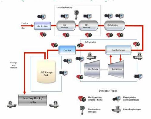
Figure 2. This simplified LNG process drawing indicates where detector technologies can be used.
