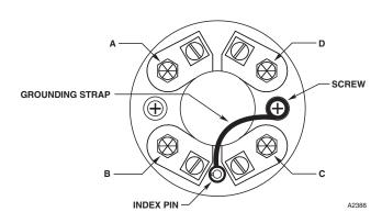
Figure 1—xWatch Terminal Block
