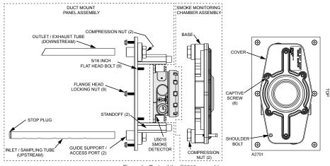
Figure 4-Parts of the Q5016 assembly
