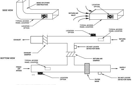
NOTE: WHEN POSSIBLE, THE DETECTOR SHOULD BE LOCATED DOWNSTREAM FROM ANY DUCT OPENING, SHARP BENDS, DEFLECTION PLATES OF BRANCH COMETONS. IF A LOCATION OPTION IS NOT POSSIBLE, LOCATE THE DETECTOR AS PAR AS POSSIBLE FROM THE OPENING BENDS, DEFLECTION PLATES, ETC.
