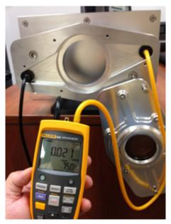
Figure 12—Manometer measurement example (Q5016 not installed)
