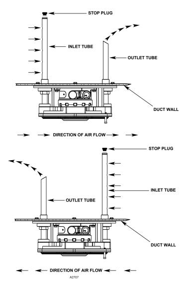
Figure 2—Tube position and orientation
