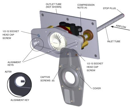
Figure 10-Q5016 Assembling front cover to plate assembly
