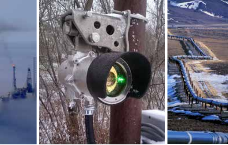
Det-Tronics FlexSight™ LS2000 line-of-sight infrared gas detector is third-party certified and is SIL 2 capable.
