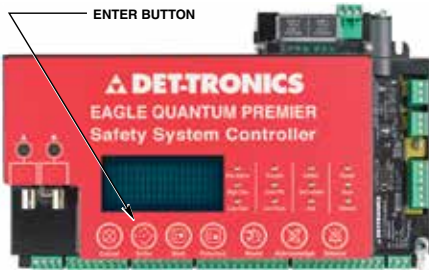
Location of ENTER Button on EQP Controller Faceplate
