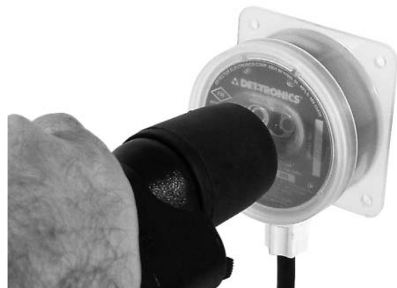
Figure 3—Testing a PM-5MP with the PSS-MP Test Set
