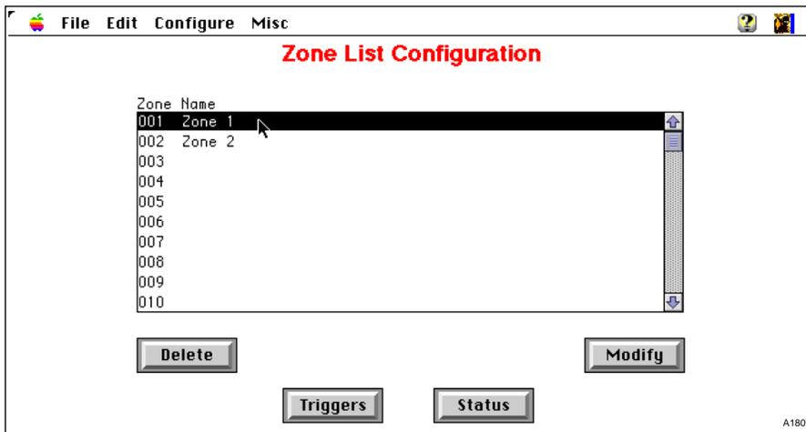
This screen displays the zone number and its name. The zone number is referenced by the zone status display and by XCMD's in graphic programming, the name can be any alphanumeric combination up to 45 characters in length. The name is used only on this screen.
