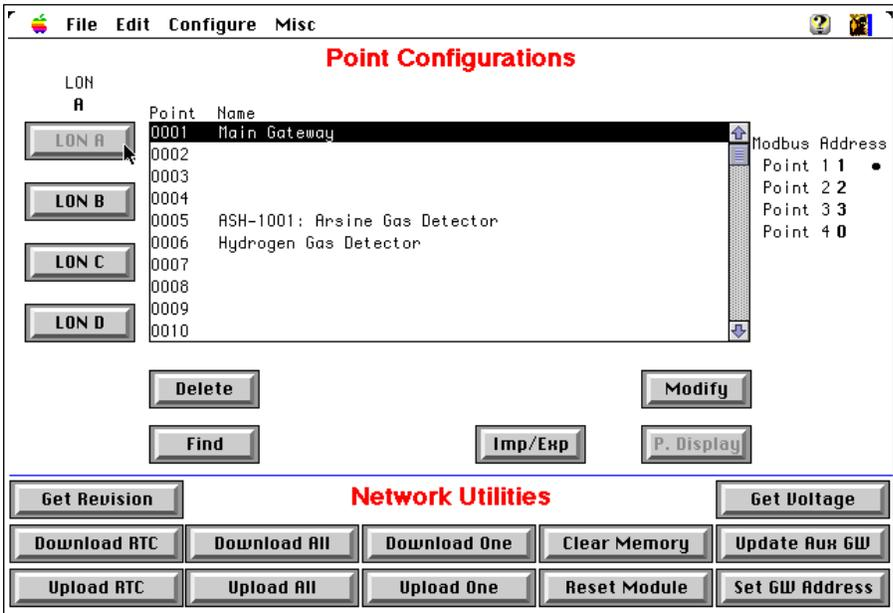
A "point" is defined as a sensing device and its communication module. Each gateway supports up to 250 points. Each point has a unique address, which is set by means of a dip switch located in the device's communication module.
