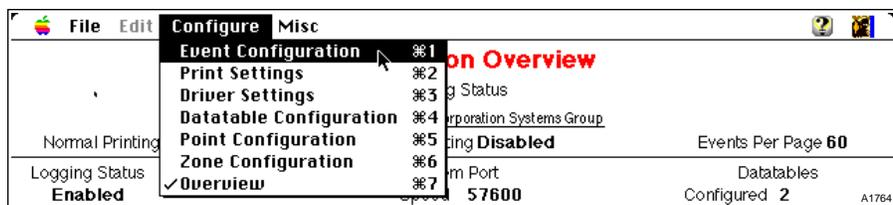
This screen is used to create events to be monitored. Event configuration defines the information required to track the status of the event and what happens should the event occur. The event configuration database is saved in the "EventsToMonitor" file in the "Detector Folder."
