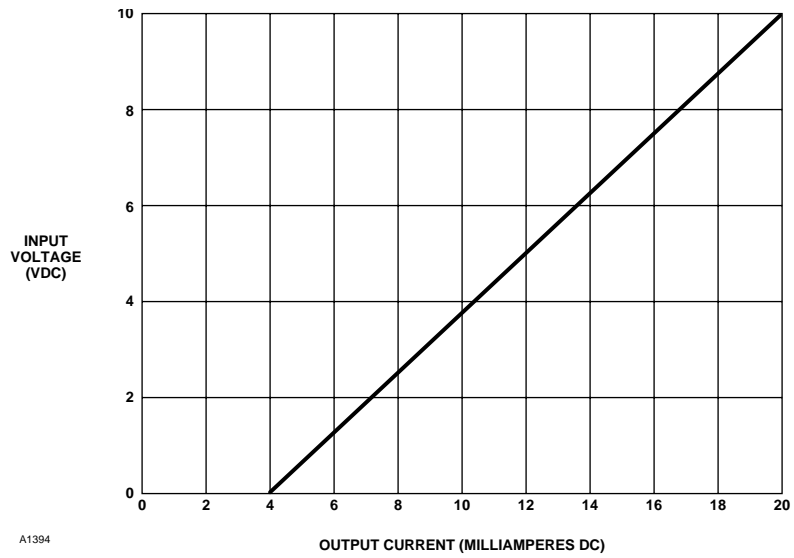
Figure A2—Voltage - Current Transfer Curve of the 4 to 20 Milliamperes Converter
