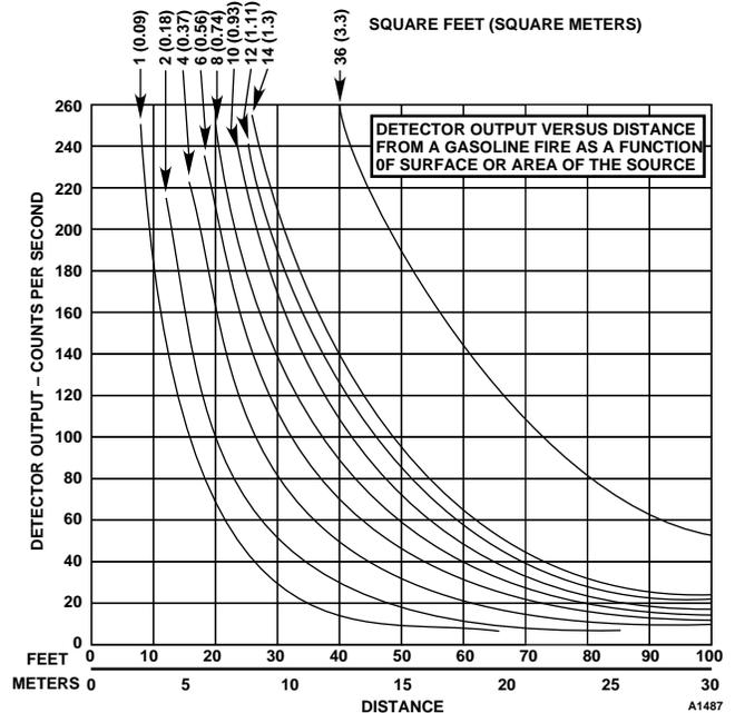
Figure 9—Sensitivity to a Gasoline Reference Fire
