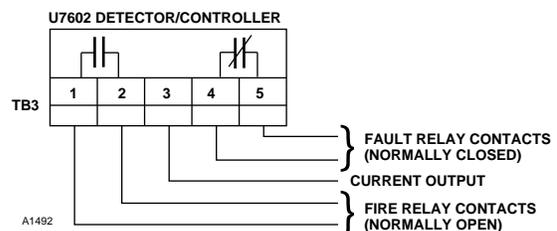
Figure 11—TB3, Relay and Current Outputs for Standard Controller Module
