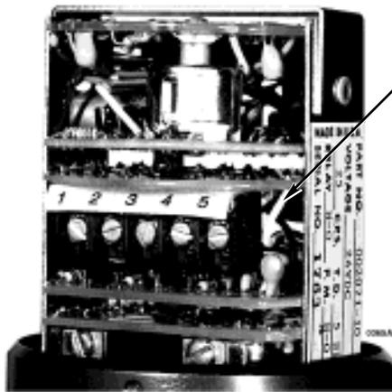
Figure 20—White Wire at the Third Circuit Board
