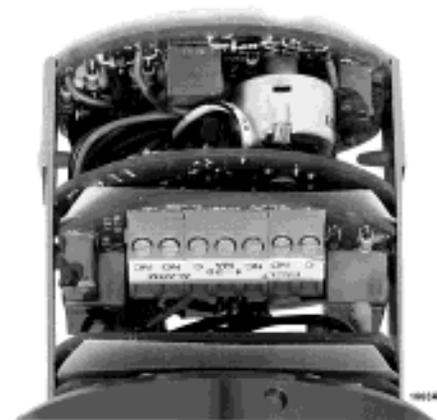
Figure 4—TB3 on Optional Form C and 4 to 20 ma Output Controller Modules
