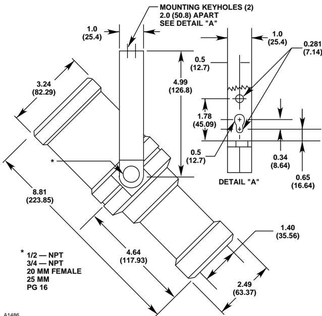
Figure 7—U7602 Dimensions in Inches (Millimeters)
