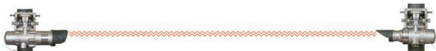
FIGURE 7. Line-of-sight gas detectors continuously monitor combustible hydrocarbon gas levels between two points at ranges of up to 120 meters. This allows a large coverage area, with the result that fewer detectors may be needed. However, a limitation of this technology is that it is unable to pinpoint the location of the leak
