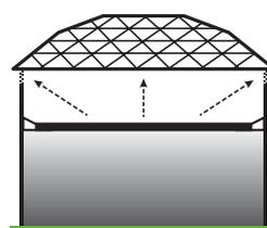
**Geodesic Dome Floating Roof Tank**
