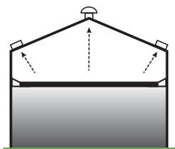
**Internal Floating Roof Tank (IFRT)**
