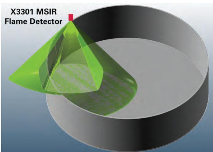
**The detection range of the Det-Tronics X3301 Multispectrum Infrared Flame Detector (FM approved to detect a 1 ft<sup>2</sup> heptane fire at 265 feet (0.09 m<sup>2</sup> fire at 80.7 meters)) allows one detector to cover a large portion of the floating roof seal along with the surface of the floating roof and, in some cases, the area outside of the tank wall.**
