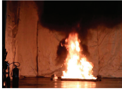
Taken at Ladd Army Airfield, Ft. Wainwright, AK, the left image shows the soot and smoke generated by traditional pan fire testing; right image depicts a new proof-testing methodology using a patent-pending Jet Fuel Flame Simulator developed by Det-Tronics.
